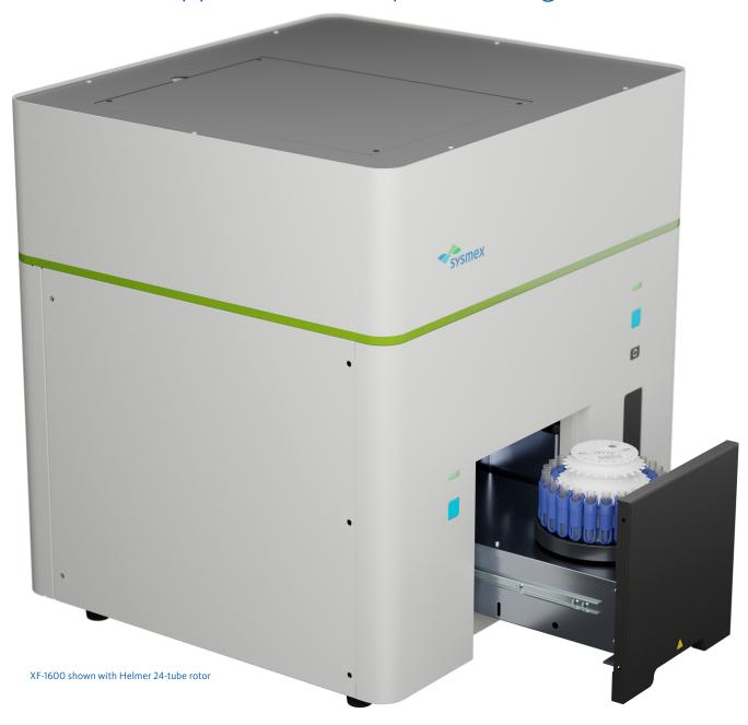
If your valuable spcimens require special attention, the XF-1600 provides unique sampling options. Single tube processing can be performed on a variety of tube sizes with selectable aspiration volumes to ensure minimal sample waste and protection against accidental sample loss. Alternatively, samples can be loaded on a Sysmex compatible rotor for automated walk-away acquisition.
