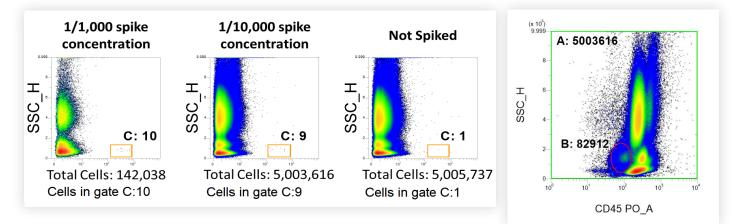
Five adjustable sample rates - from 5  $\mu$ L/min to 120  $\mu$ L/min - provide flexibility for all sample types, titer levels and cell concentrations. At high sheath velocity, fast data acquisition rates – up to 50,000 events per second - reduce the overall sample acquisition time while maintaining sensitivity required for rare event analysis.
